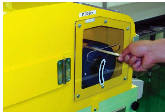
Using chopsticks to demonstrate getting caught in a V belt
