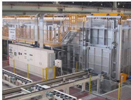
YKK AP INC. Shikoku Plant We are switching from heavy oil and kerosene to LNG as part of a medium-to long-term goal. By switching to LNG in our extrusion heat processing furnaces, boilers, air heating furnaces, melting furnaces, holding furnaces and other equipment between 2007 and 2011, we will be able to reduce CO 2 emissions by 8,000 tons.
